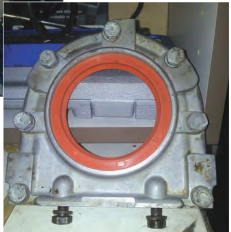
Picture 4: New seal fitted to housing, top bolt to have a copper washer
