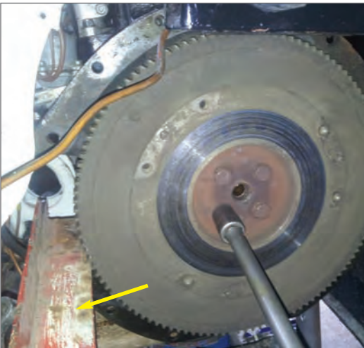
Picture 2: Preventing the crankshaft from turning
