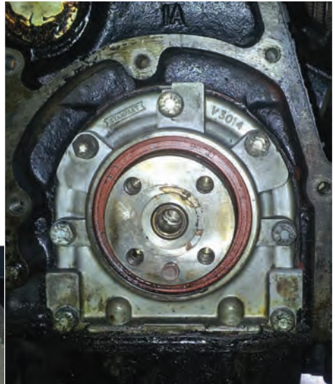
Picture 3: Old leaking seal in position on engine
